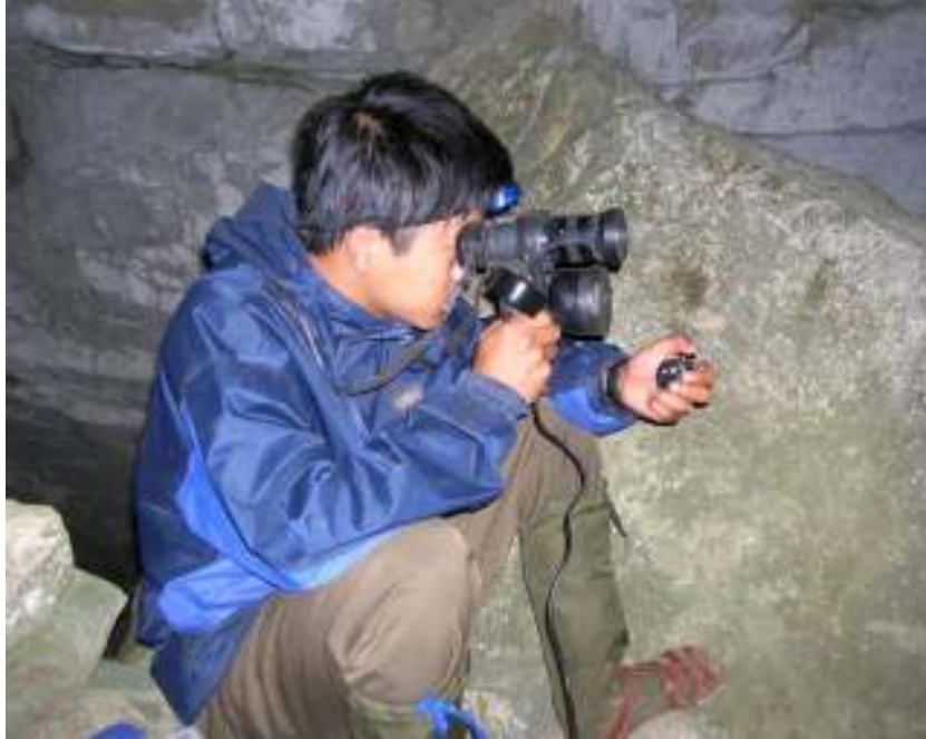
Fig. 4: Emergence count using a night vision device (with an infra-red spotlight) and manual hand counter.
